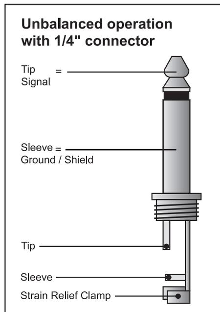
*Fig. 5.1: Wiring of a mono 1/4" plug*
